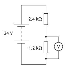
The reading on the voltmeter is
