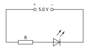
The voltage across the LED is 2.2 V. The current in the LED is 10.0 mA. The resistance of resistor R is
