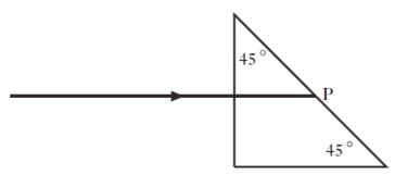
The glass has a critical angle of 40  $^{\circ}$ .
