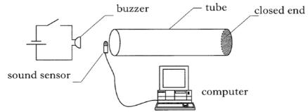
The buzzer produces a short pulse of sound. At the instant the buzzer is operated the computer starts to record the output voltage  $V_{\rm o}$  of the sound sensor.
