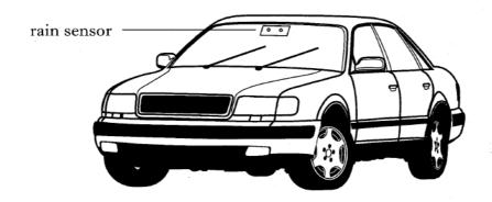
The rain sensor contains an LED which emits a beam of infrared radiation inside the car. In dry conditions this beam travels through the glass and is picked up by a detector as shown below.
