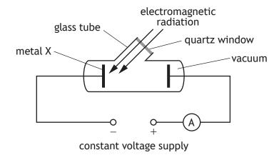
(a) The frequency of the electromagnetic radiation is varied. The maximum kinetic energy of the photoelectrons emitted from metal X is determined for a range of frequencies.
